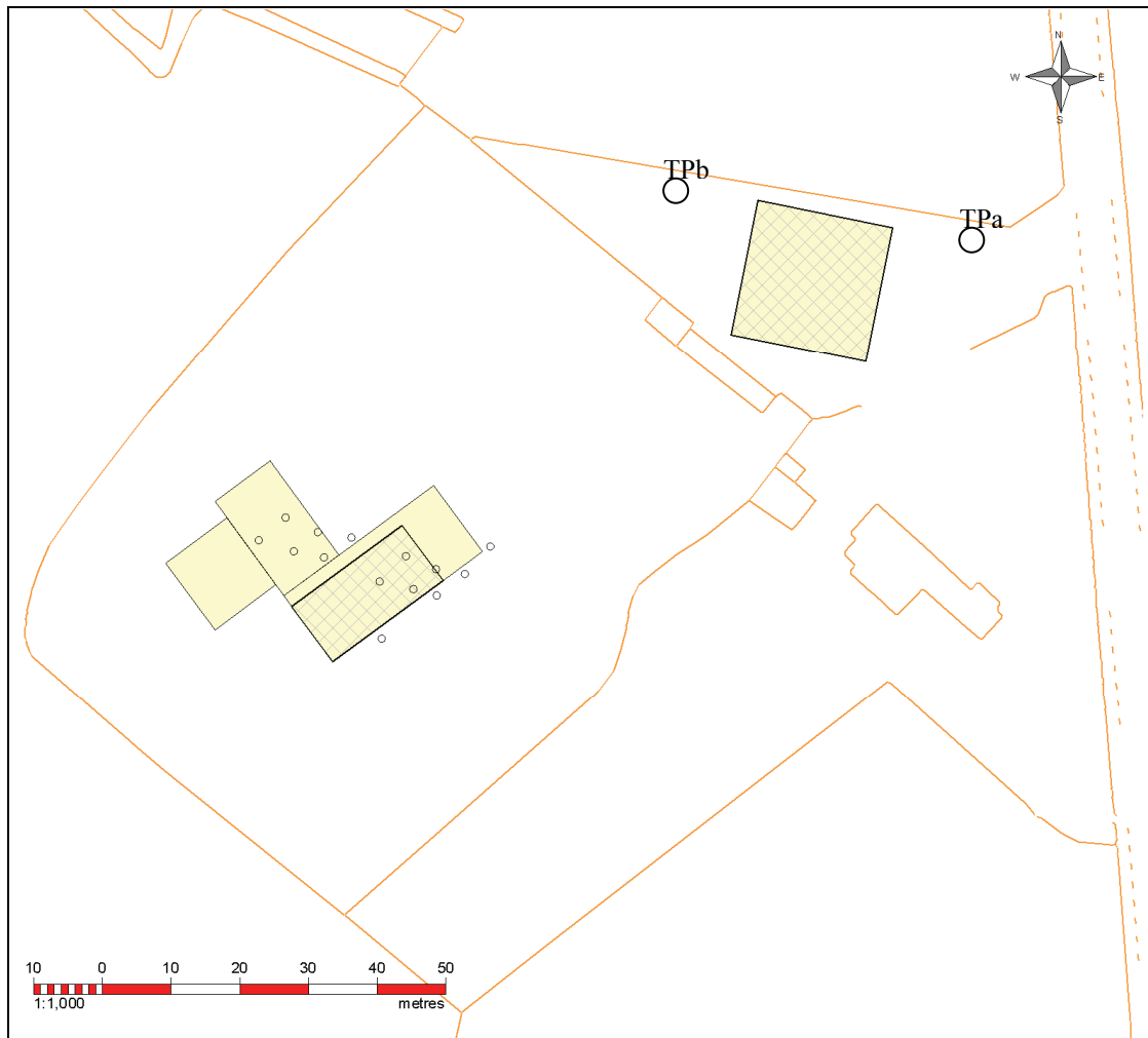
Location plan: Survey areas with Clayhithe Road to the east. (Resistivity survey areas solid, Magnetometry areas crosshatched, trees circles)
