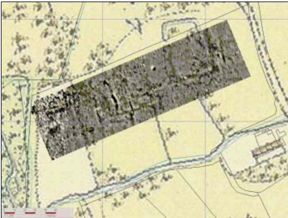
Magnetometry survey superimposed on Withers' map with current features.
