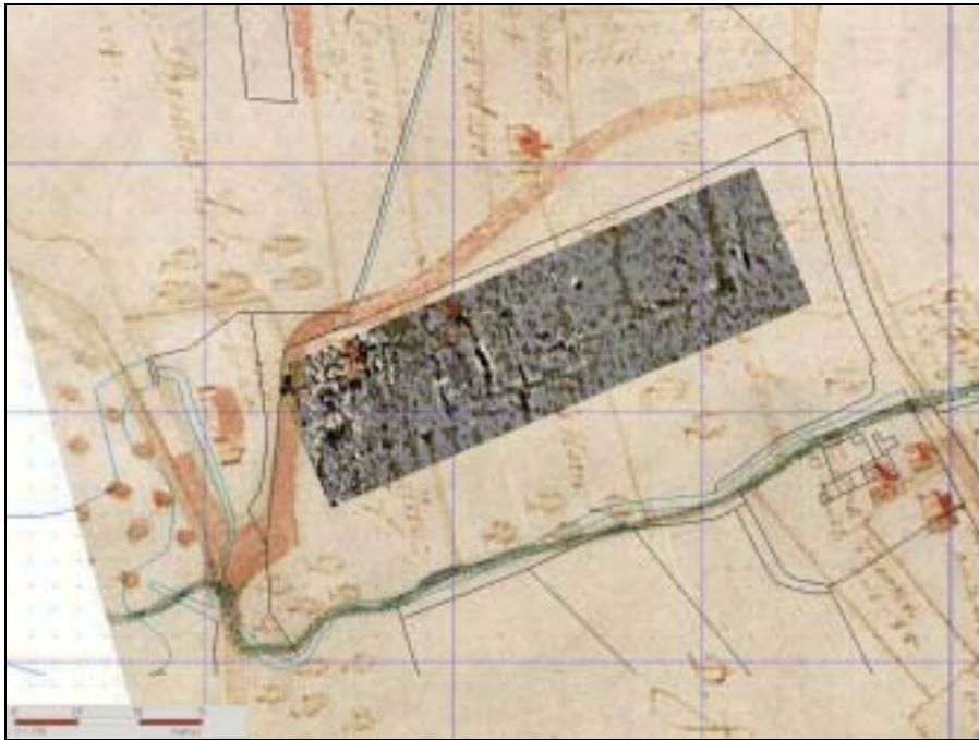
Magnetometry survey superimposed on Hare's map with current features.
