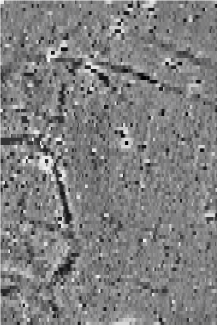
Magnetometry 60 m x 90 m range +3 to -3 nT
